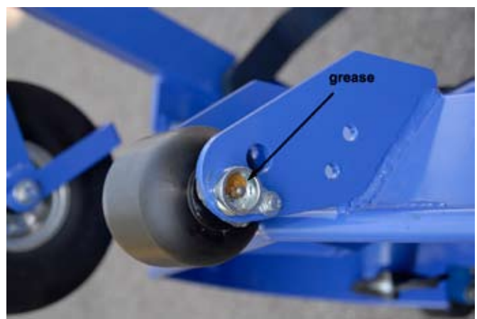
fig 24 Anti scalping rollers are mounted on greasable shafts.
