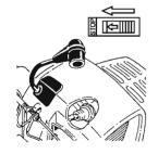
3) Disconnect spark plug cap before you work on the unit or leave it unattended.
