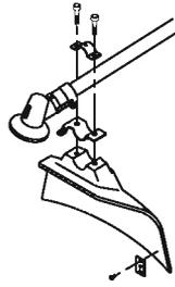
**GB ● Installation of cutting attachment guard**
