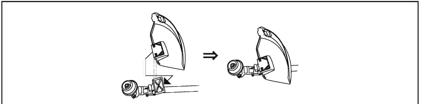
**GB ● Installation of cutting attachment guard**
