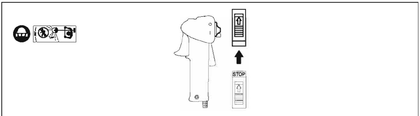
GB Turn the engine switch to the "STOP" (O) position.
