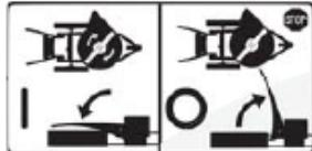
• **Engine Start/Stop:** informs the user about the operating mode of the engine stop lever. With the lever pressed, the engine is ready to work. Release the lever and the engine stops immediately.
