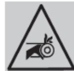
• **Dragging or locking of moving elements warning:** Informs the operator of residual risk beneath the belt cover.
